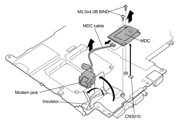
Figure 4-39 Removing the MDC
